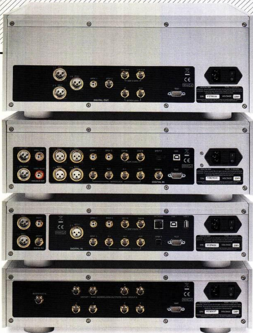
ABOVE: Connections include S/PDIF (BNC/RCA), AES and dual-AES (XLR) supporting LPCM/DXD to 352.8/384kHz and dCS-encrypted DSD (as 1-bit/2.8MHz) plus 44.1kHz and 48kHz-centric wordclocks (also on BNC). The Upsampler adds network and USB B
