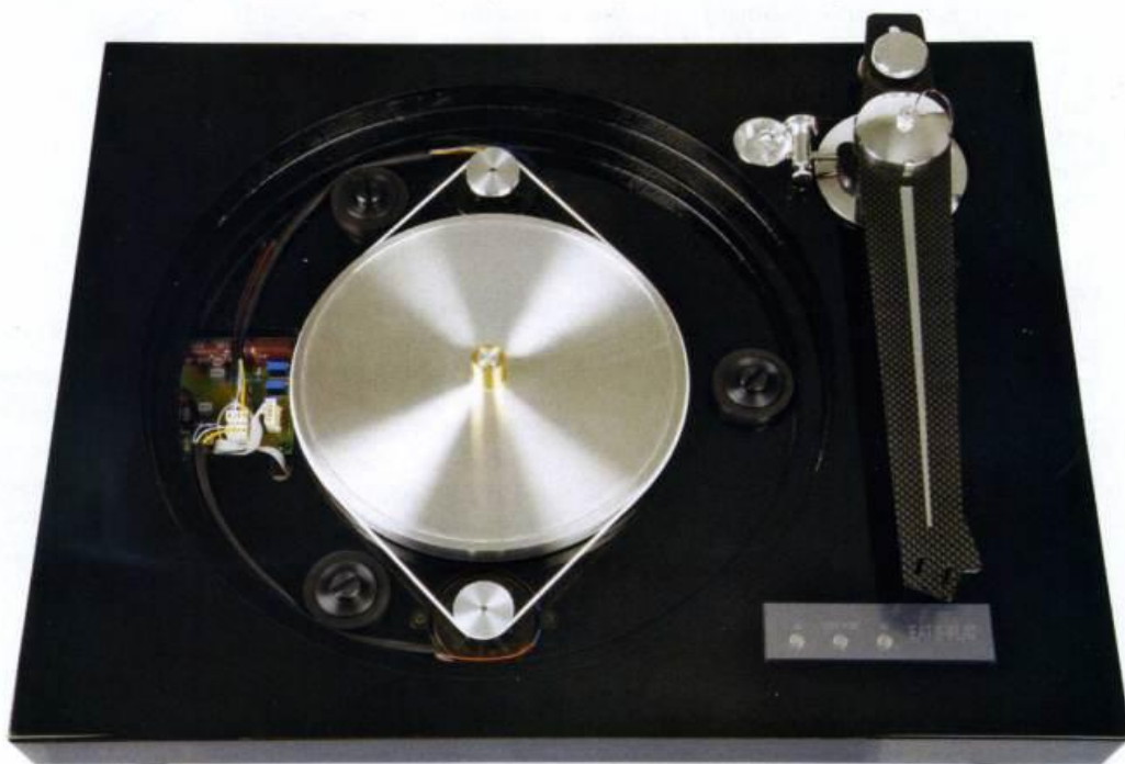
RIGHT: Unlike its siblings, the E-Flat hides its two motors and belt, visible only with outer platter removed. Assembly is straightforward, but care is needed with the tonearm
