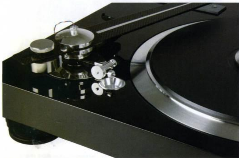
ABOVE: No challenge to those who know unipivots, but read the instructions when setting it up; exposed wires, though, tend to detract from the look of the arm
