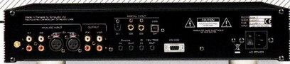
ABOVE: At the rear are balanced and unbalanced analogue inputs and, if the unit has the optional built-in DAC, a set of digital inputs including Toslink optical, two coaxial (S/PDIF) connections and USB. The RS-232 port allows for firmware updates
