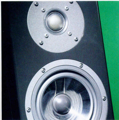
ABOVE: A hand-coated silk domed 28mm tweeter sits above the 150mm mid driver, on a 40mm Medite baffle
