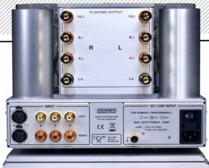
ABOVE: There are four line inputs, one balanced (XLR) and three single-ended (RCA). Output transformer has speaker binding posts for 4, 8 and 16ohm loads
