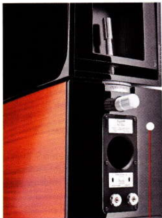
• The Kiss cabinet's pivoting mechanism, as seen from the back of the speaker.
